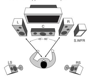
After connecting the speakers, set the speaker installation information properly. You can use Quick Speaker Setup for it (see page 18).
